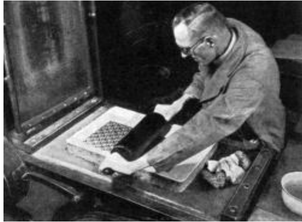
Top - An inked roller is worked to and fro over the dampened surface.
