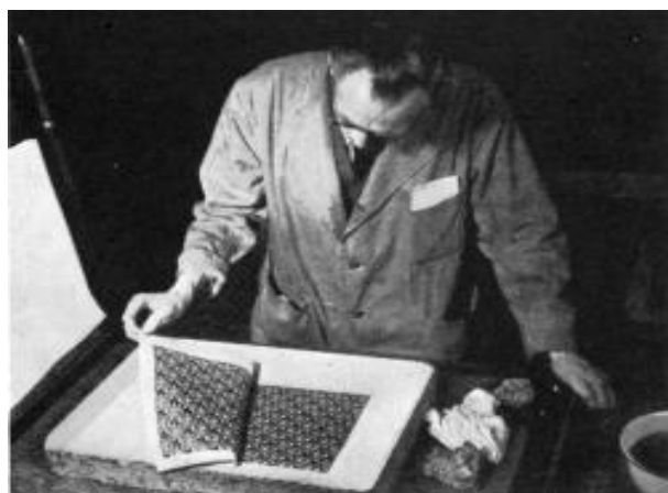
Right - The tympan is lifted and the print removed from the stone.
