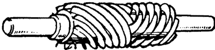
of the blade. There are two helixes meeting in the middle of the cylinder. As the blade spins, the blades stretch the skin both lengthways and sideways, and in the process remove the majority of creases that are present in the skin.
