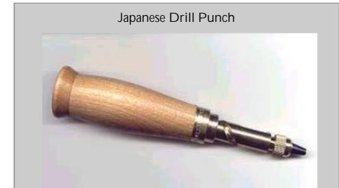
This very clever product is now available from Hewit's. The brass chuck holds one of the 7 drill bits supplied with the Punch. Pressure exerted downwards, causes the bit to spin, drilling through paper and board without 'snagging'. Excellent for drilling through paper, leather, board, etc. The drill comes with 7 bits - 1.0mm, 1.5mm, 2.0mm, 2.5mm, 3.0mm, 3.5mm and 4.0mm. Spare sets of Bits are also available:
