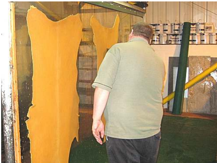
Most of our calfskins and a proportion of our goatskins are dried on large sheets of glass.
