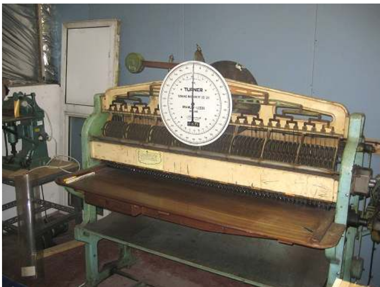
Our pin-wheel measuring machine
