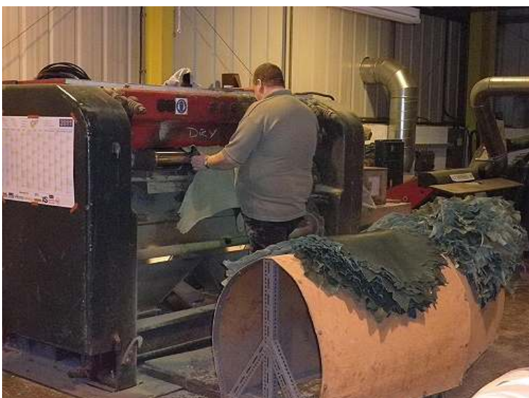
Chieftain Goatskins are shaved to the correct substance.
