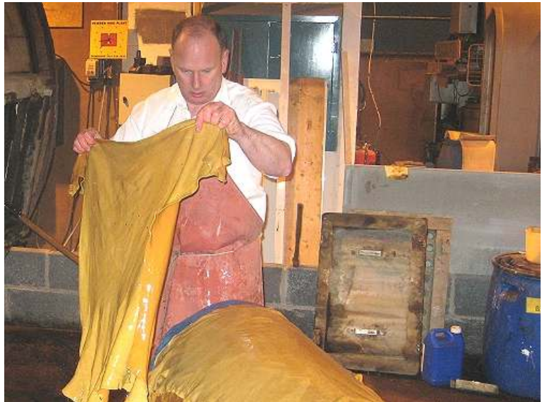
Dyed goatskins, are removed from the drum and are being 'horsed' up ready to be dried.
