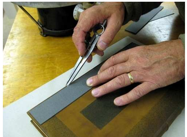
A strip of millboard and dividers are used to establish the position of the double line around the edge of the board.
