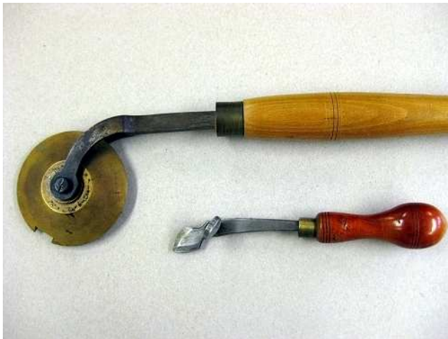
Blind lines around the three rectangles can be produced with either a two line fillet or adjustable leather creaser.
