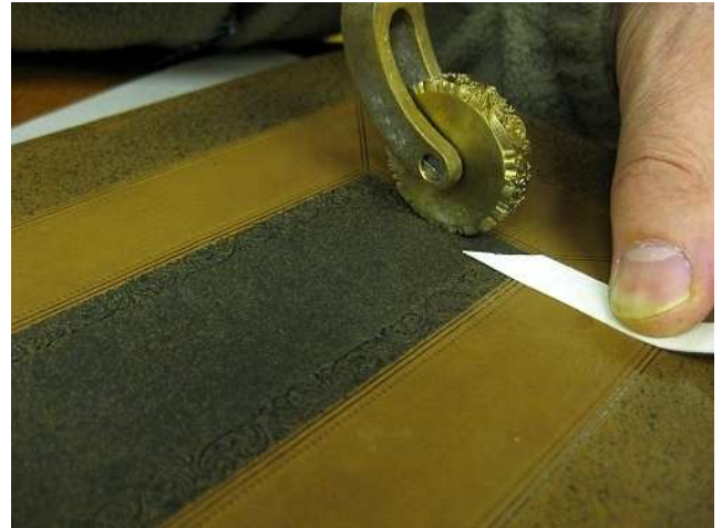
A decorative roll is used around the inside perimeter of the darker centre panel and the corners mitred using a strip of vellum with the end cut at forty five degrees.
