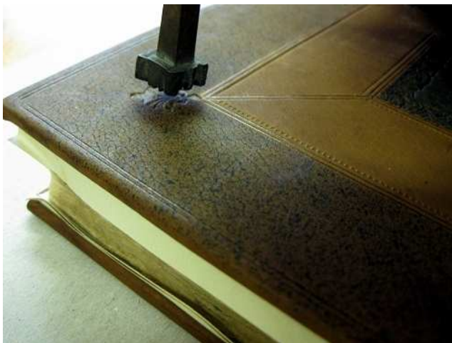
An appropriate centre tool is impressed into the leather at each outer corner of the centre frame.
