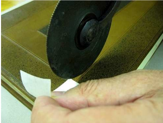
A strip of vellum held in position provides a stop for the roll.
