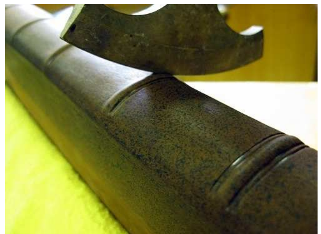
A warm two line pallet is impressed on each side of the raised bands to give a double blind line.
