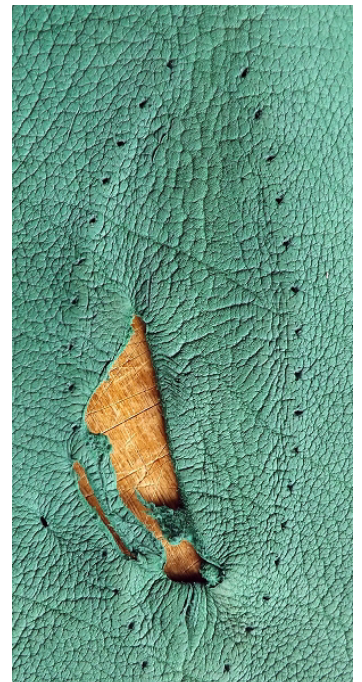
Bottle tanned calfskins ca. 1950, showing the stitching around the edges and also around a hole in the skin
